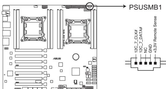
**Z9PE-D8 WS Power supply SMBus connector**
